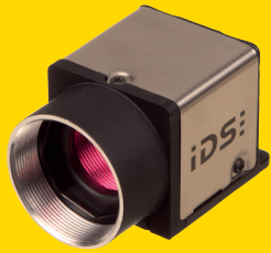
IDS HIGH SPEED USB 3 COLOUR CAMERA 1280x1024 @ 60fps
